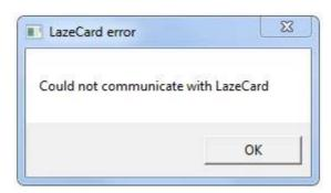
After you have confirmed this notification by clicking on *OK* you are still able to use the "XS Designer" in the simulation mode and edit your markings. Nevertheless the start of a marking process is only possible if the LazeCard which is integrated in the Lasebox is able to make a functioning connection to the computer.
