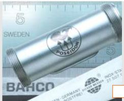
The electrolytic marking is based on an electrochemical reaction. The exact image of a stencil is reproduced on the surface of any conductive material through the reaction of the electrolytic solution and a low current. The design of the stencil is not limited in any way.
